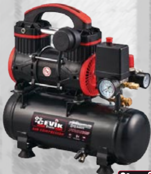
PRO6XS Ref. A066072 230V-50Hz-1HP-6l-156 l/min- 8 bar- 69dB Sin aceite
